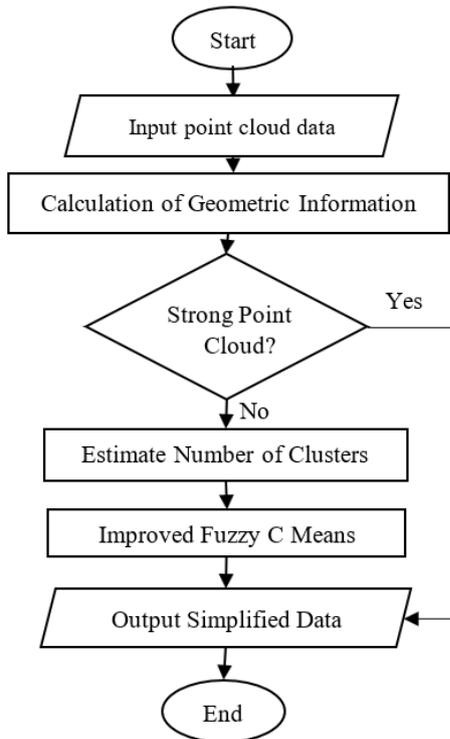
Figure 1. Flowchart of the developed point cloud simplification algorithm.
